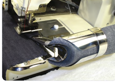
Makina / Machine : •Kemer Makinası Waistband Machine
