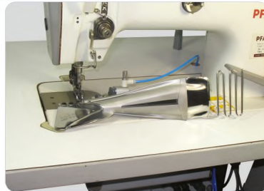
Makina / Machine : •Ayak Transportlu Düz Makina Bottom - Top Feed Lockstitch Machine
