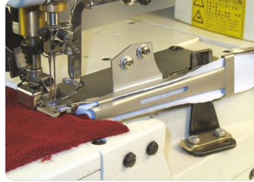
Makina / Machine : •Bant Reçme Makinası Coverstitch Machine for Tape Binding
